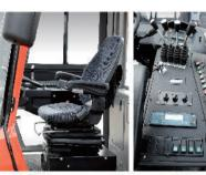
■ Moveable dashboard Most reasonable relative position is set between dashboard and seat SIP point through optimized ergonomic and multiple test. Dashboard and seat can be moved together to meet different driving
