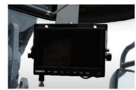
Rear vision system (optional) truck real time rear view can be displayed when backward.
